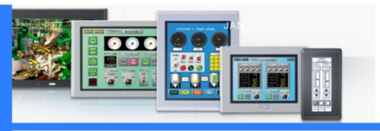
ALTHOUGH HMI IS THE MOST COMMON TERM FOR THIS TECHNOLOGY, IT IS SOMETIMES REFERRED TO AS MANMACHINE INTERFACE (MMI), OPERATOR INTERFACE TERMINAL (OIT), LOCAL OPERATOR INTERFACE (LOI), OR OPERATOR TERMINAL (OT). HMI AND GRAPHICAL USER INTERFACE (GUI) ARE SIMILAR BUT NOT SYNONYMOUS: GUIS ARE OFTEN LEVERAGED WITHIN HMIS FOR VISUALIZATION CAPABILITIES.
