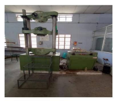
21. Loading Frame / Hydraulic remote type jack, hydraulic power pack with hose (100KN), control panel with 50 tonne capacity, load cell (100 KN) with digital indicator  $\,$
